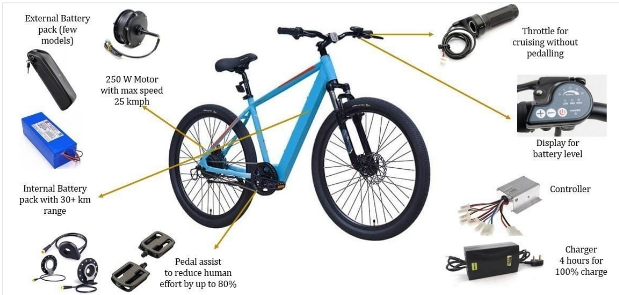
Figure 5: Components of electric bicycle
